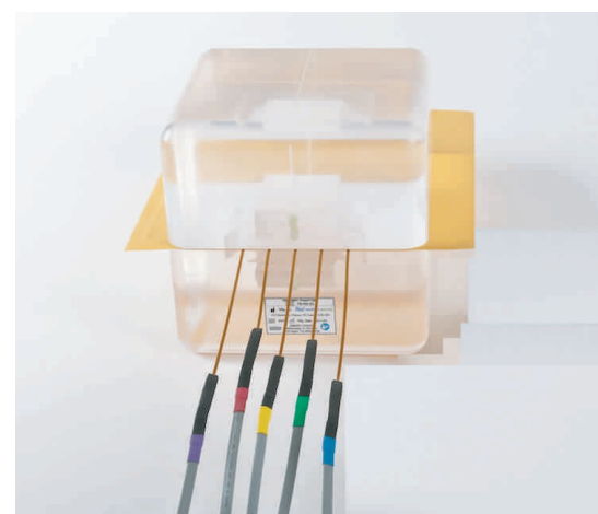
A film placed between the two sub-phantoms using MOSFETs dosimeters for IMRT plan.
