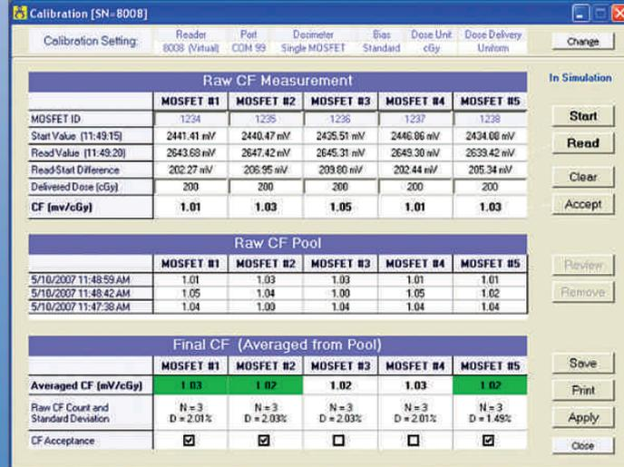
Calibration is made even easier using the mobileMOSFET Software Calibration Module along with the Calibration Jig. The jig allows for consistent placement every time while the software helps you determine your calibration factors with a few clicks of your mouse. The result is consistent and reproducible calibrations.
