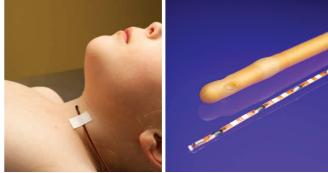
MOSFET dosimeters are small, light-weight, unobtrusive, and versatile. Pictures above show the small size of the microMOSFET, a high-sensitivity MOSFET being used to measure scatter dose to the thyroid, and the Linear Sive Array for use in brachytherapy.
