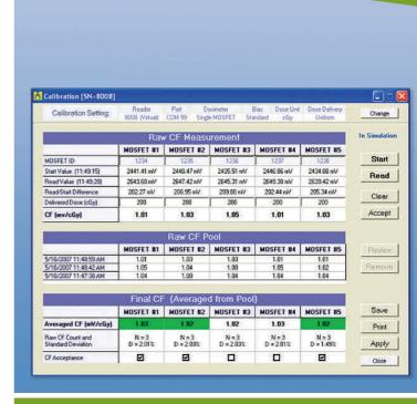
Calibration Module  $\,$  along with the Calibration Jig . The jig allows for consistent placement every time while the software helps you determine your calibration factors with a few clicks of your mouse. The result is consistent and reproducible calibrations.
